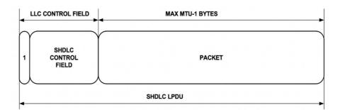
Figure 7.11: LPDU structure of the LLC layer of type SHDLC
