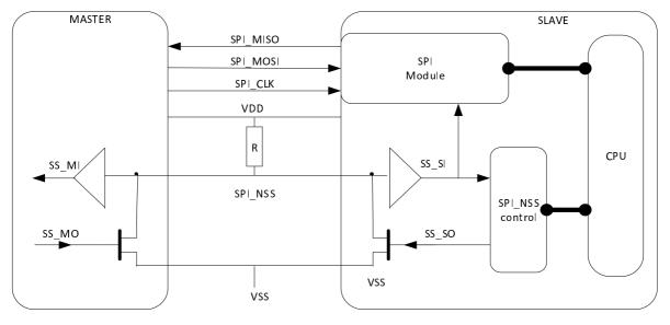
Figure A.2: SPI interface with 4 wire
