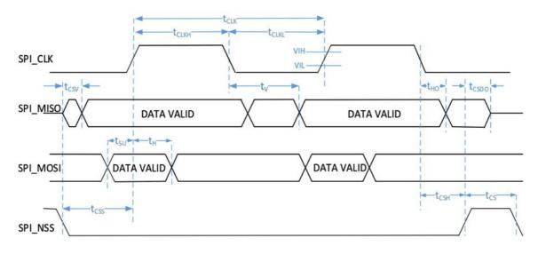
Figure 6.3: SPI timing diagram
