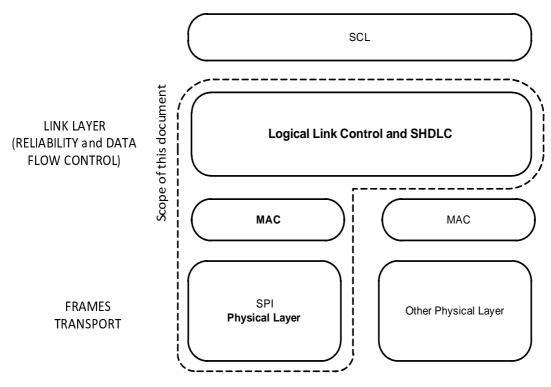
Figure 5.1: Protocol stack for SPI Interface
